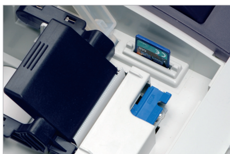
Slot for the SD MEMORY CARD to store all data in compliance with 2018 fiscal norm
